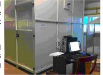
The standard specifies a method of measurement of smoke density of cables. Part 1 specifies the test apparatus and Part 2 specifies the test procedure.
