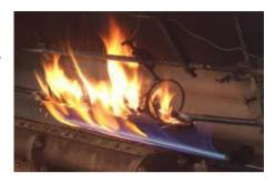
IEC 60331-11 ed1.01 Consol. with am1 (2009-07) – Part 11: Apparatus – Fire alone at a flame temperature of at least 750°C.
